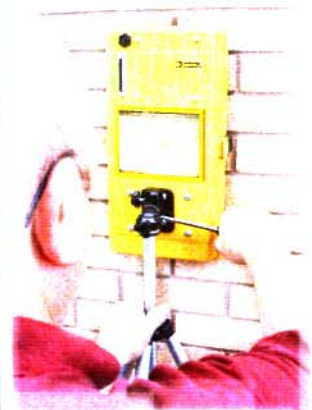
Cambridge Consultants' second-generation Prism 200 radar can 'see' through thick walls, and distinguishes individual targets with different colors
